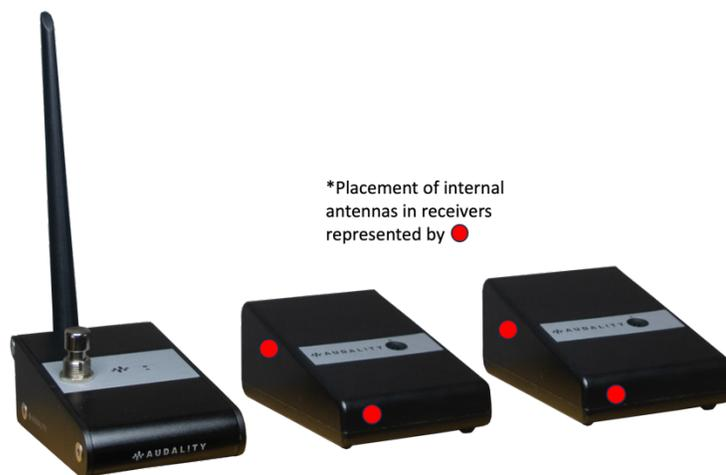
\*Placement of internal antennas in receivers represented by ●
